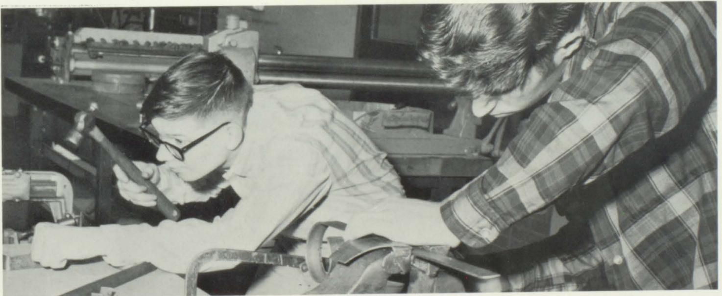
Below: R. Letarte and J. Dumbrozio cut, flare, and bend scrolls in ornamental iron.
