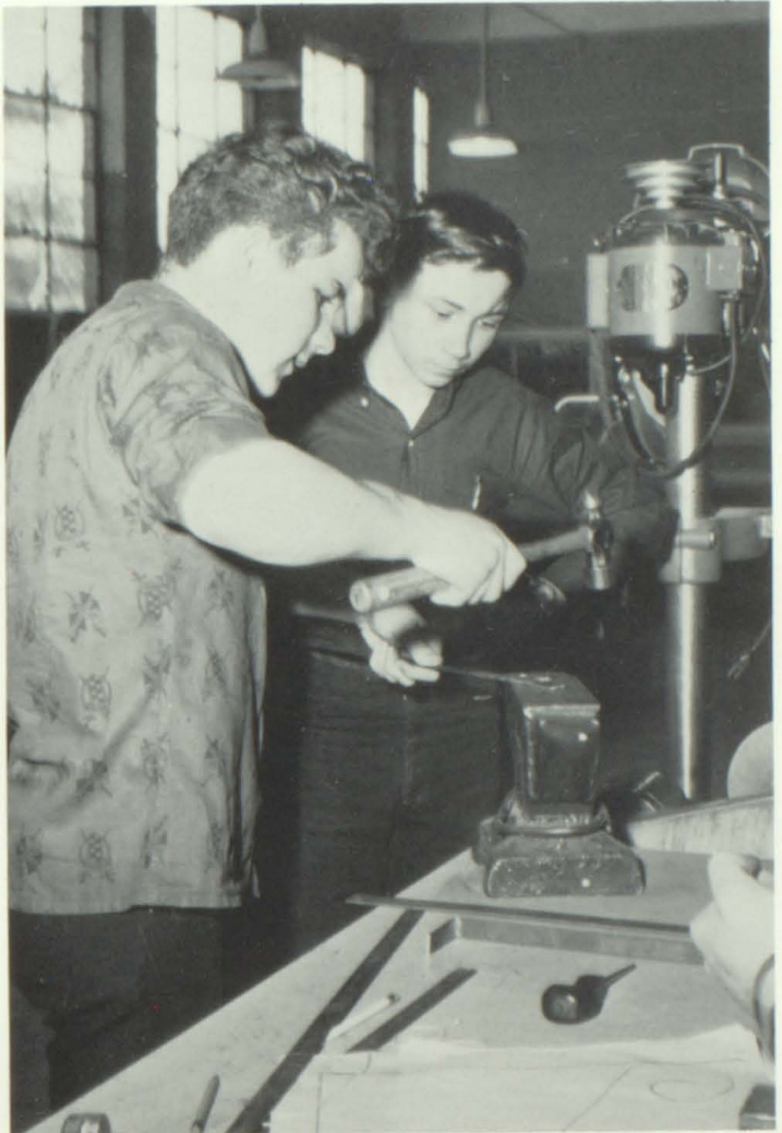
L. Jones and D. Parker flare mild steel as a part of a unit in ornamental iron work.
